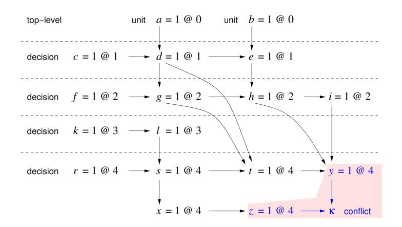
UIP = *articulation point* in graph decomposition into biconnected components (simply a node which, if removed, would disconnect two parts of the graph)
