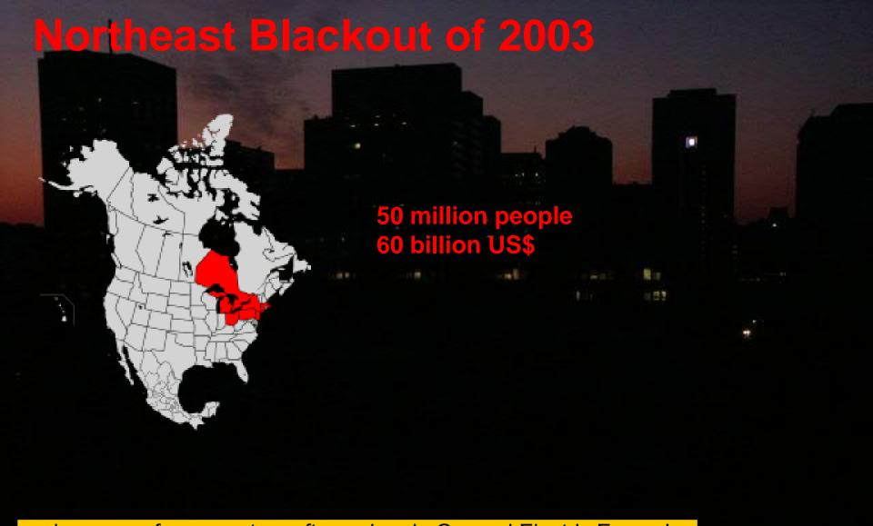
... because of a computer software bug in General Electric Energy's Unix-based XA/21 energy management system that prevented alarms from showing on their control system. This alarm system stalled because of a race condition bug.
